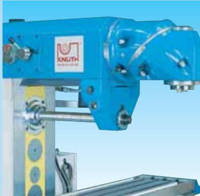
Horizontal milling with rigid outer arbor support
