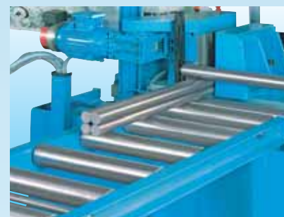
A bundle vise is provided for cutting entire material packs to length
