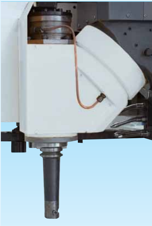
Horizontal spindle position with optimum chip exhaust for improved surface quality, and longer tool life provide increase production quality and lower costs
