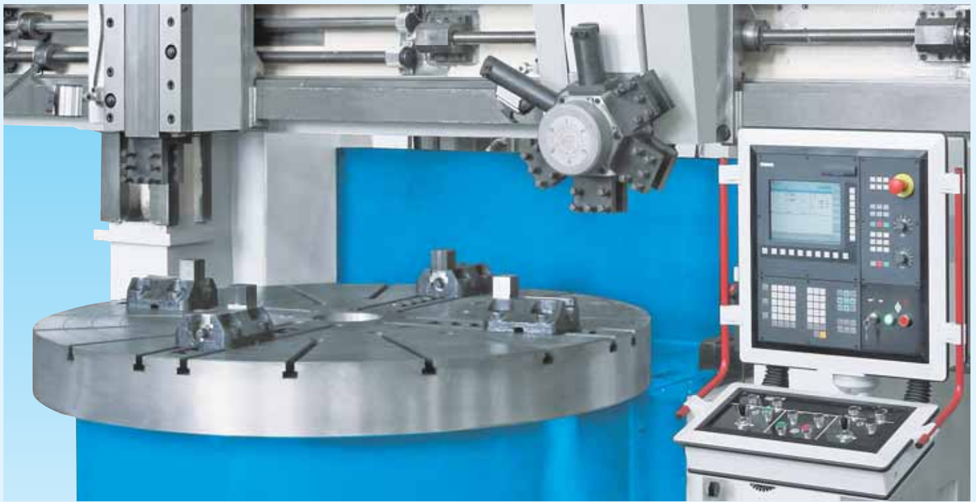
6-station tool turret provides high degree of automation and quick changing at the CNC controlled work unit
