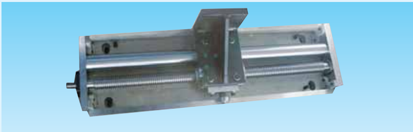
preloaded ball screws for zero-backlash positioning of the rear stop
