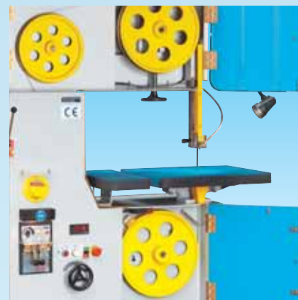
optimum blade tension via hand-wheel
